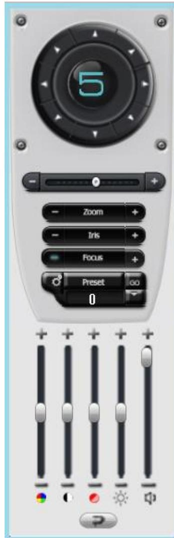
Equipment can achieve to PTZ control function through RS485 external connect with PTZ device, also control the run speed of PTZ ,test the Zoom , adjust focus and Iris , c preset , and brightness contrast etc.
